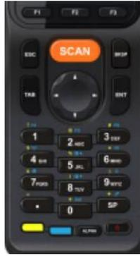
To suspend and resume operation, press the Power button. You may also press the front Scan key to wake a suspended device unless the battery door has been removed and replaced.
