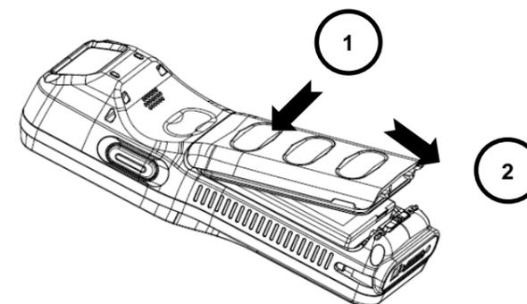
3. Replace the battery door to start from top to bottom door's lock downwards.
