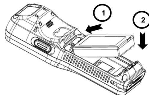
2. Insert the battery well with the battery cells facing top.
