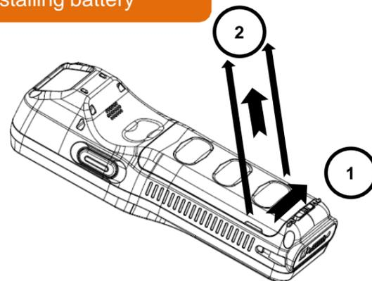
1. Remove the battery compartment door by moving the Battery door's locks Push.
